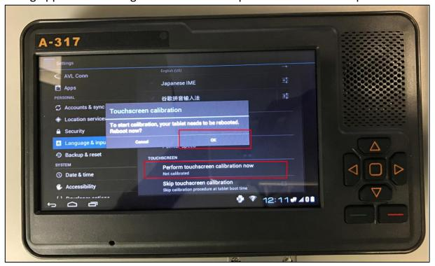
6. Once the MDT3300 restarts, follow the on-screen calibration instructions. *Use a stylus to get the most accurate results*. Once the calibration steps are complete, the MDT returns to the home screen and is ready to use BSM applications.
