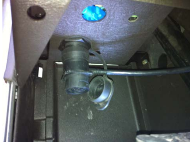
Figure 2-4 Connecting a Locator mounted outside the dashboard
