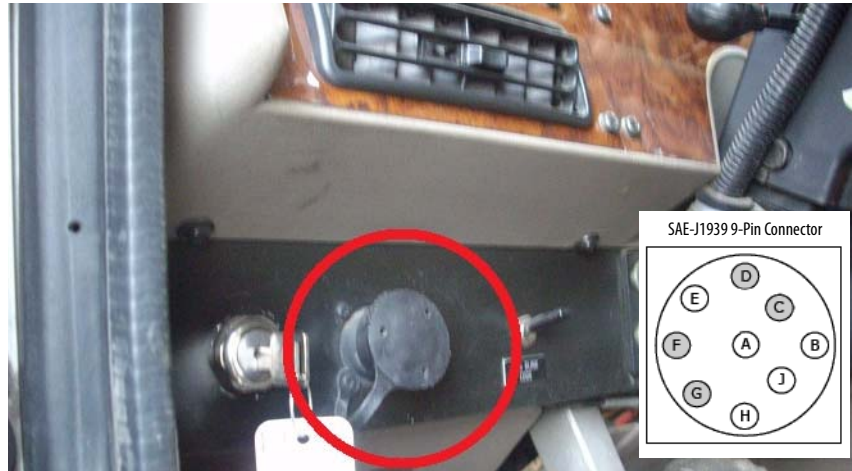
Figure 2-2 Vehicle SAE-J1939 9-Pin Connector
