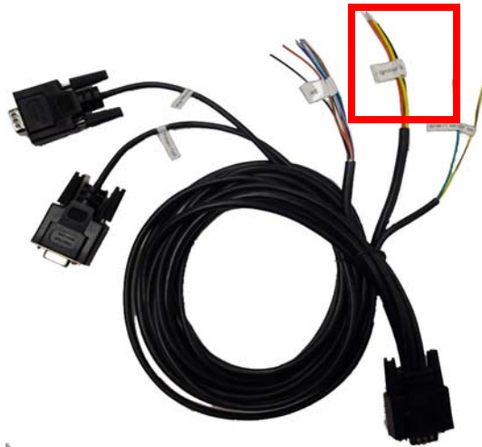
Figure 5-1 Telemetry wires on the Locator's cable
