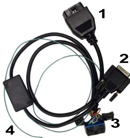
Figure D-3 OBDII Y-cable (1) male 16-pin J1962 connector (2) DB15 serial connector (3) female 16-pin J1962 connector (4) Fail-safe wire
