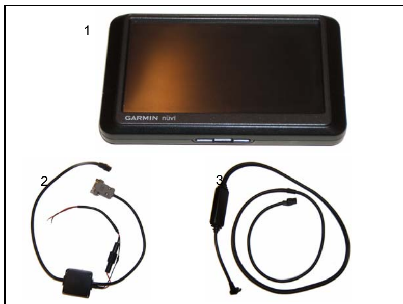
Figure H-11 Shown: Garmin Nüvi (1), custom cable lower half (2), custom cable upper half (3). Not shown: mounting bracket and suction cup.
