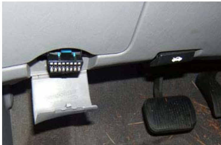
Figure D-6 Example of an OBD connector (female 16-pin J1962) in the access panel after Locator and OBD installation
