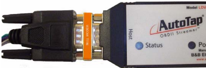
Figure E-10 OBDII Gateway with null-modem adaptor and Locator cable attached
