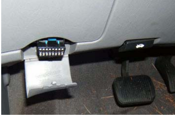
Figure E-11 Example of an OBD connector (female 16-pin J1962) in the access panel after Locator and OBD installation
