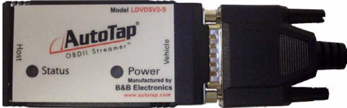
Figure E-9 OBDII Gateway with OBDII Y-Cable attached
