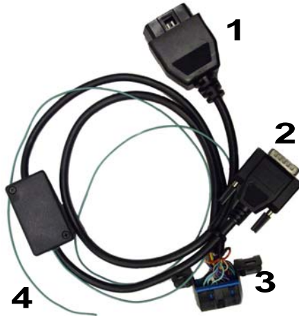
Figure E-8 OBDII Y-cable (1) male 16-pin J1962 connector (2) DB15 serial connector (3) female 16-pin J1962 connector (4) Fail-safe wire
