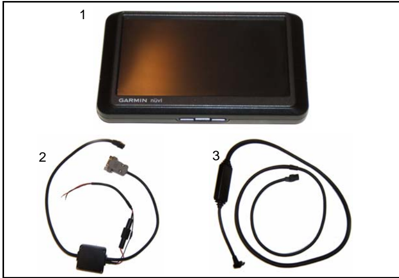
Figure C-7 Shown: Garmin Nüvi (1), custom cable lower half (2), custom cable upper half (3). Not shown: mounting bracket and suction cup.
